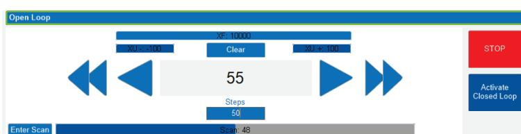
The theoretical position in steps number is displayed at the center (for Open Loop Stage).
